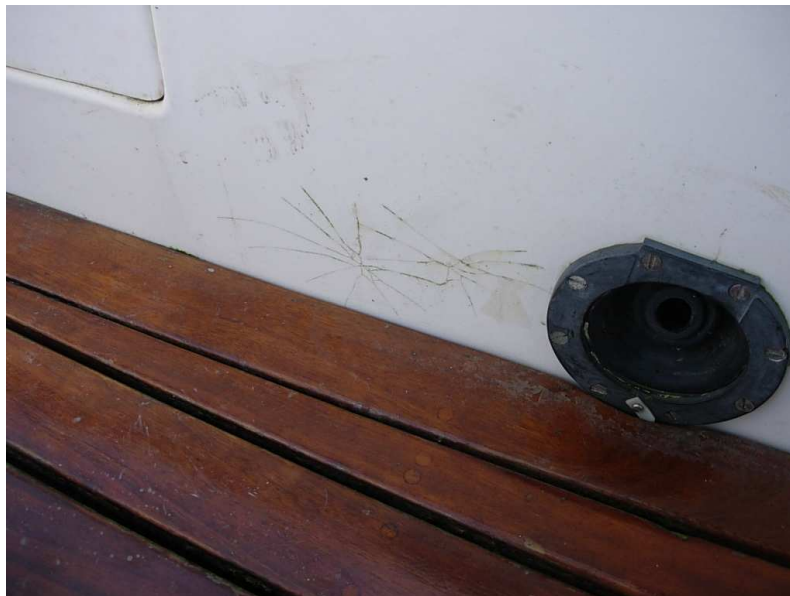
Figure 2 Areas of crazing in cockpit well to port.
